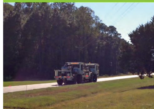
The small-scale UNIVIB vibrator generated significant force energy penetration at low frequencies for deep target data acquisition.
